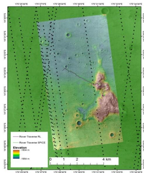
**Figure 2. MER-A traverse from optical navigation (labelled RL) and from the original SPICE kernels after co-registration of HiRISE (insert) with HRSC (background). Individual MOLA footprints are shown to highlight the difficulty in finding common MOLA-HiRISE points.**
