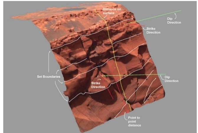
can be used as landmarks, i.e. it is possible to interactively fly to the corresponding locations. This set of interactive tools enables planetary scientists to map geological surfaces and rock layers over large areas in a quantitative framework. Overall, they are able to construct digital models of rock outcrops that assist in identification of ancient sedimentary environments that may have been habitable.
