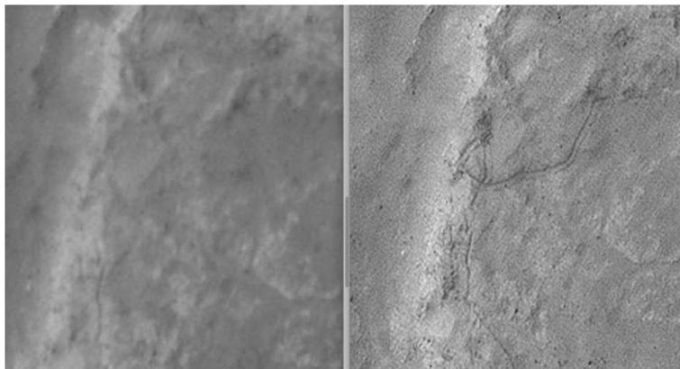
Figure 2. MER-A Homeplate: 25cm HiRISE (left) and super-resolution 5cm imagery generated from a stack of 8 inputs
