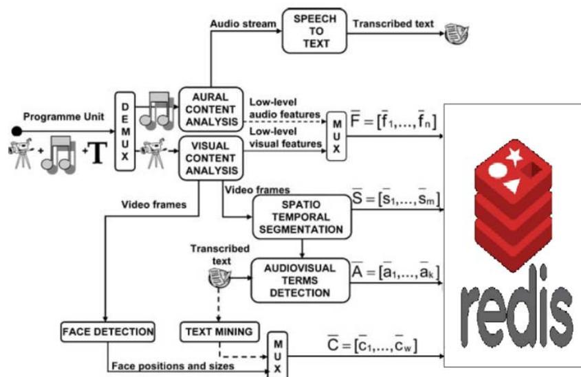
Figure 1. Architecture for multimodal frame-based feature extraction and storing.
